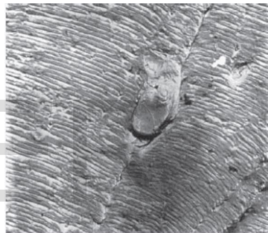
Fig 1 Typical striations around sample due to welds
