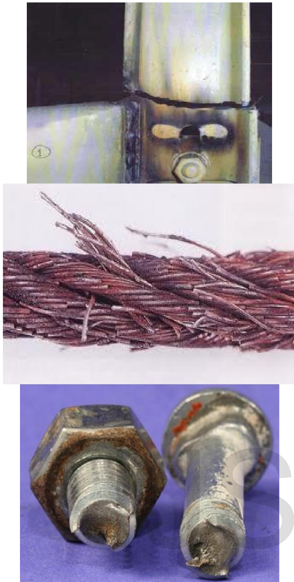
Fig 3 Component failed due to Fatigue Failure Example
